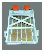
Once setup is achieved with favorable steady-state conditions, operation is as simple as starting the motors with the flip of a switch, and letting the screen do its job without further concern. One of the greatest benefits of operating RMB KNOVATECH dewatering Screens is having the ability to adapt to each plant's unique material by combining the adjustable motor force with the adjustable bed tilt.
