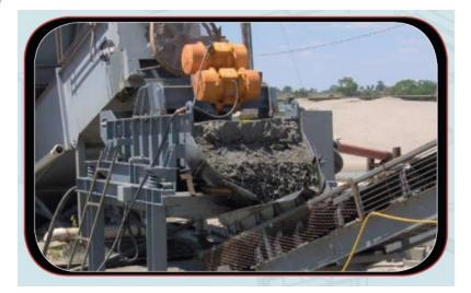
Each unit receives a high percentage of water-saturated fine material and produces a dense, compact cake that rides up the belt and forms a pile with no runoff or water pools. This provides a dry, transportable product that can be sold in a short period of time.
